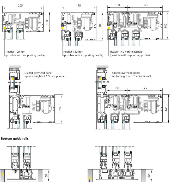
Full-lenght bottom rail integrated in the floor (for increased safety and stability), bottom rail with drainage optionally available
